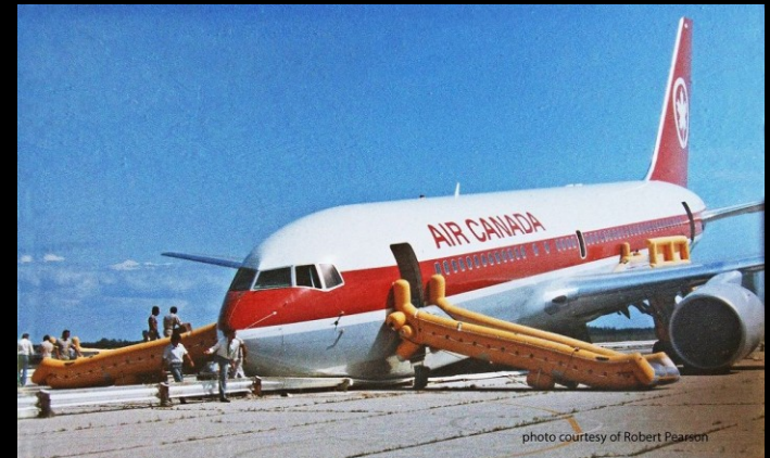
Gimli Glider Ran out of fuel @ 40,000 feet Wrong units for fuel calculation
