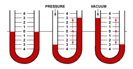
U- Shaped tube connected to apparatus Measures difference in column height as pressure
