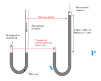
Measure height mercury (P) Measure Volume (V)
