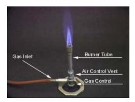
The Bunsen Burner burns natural gas (primarily methane, CH<sub>4</sub>). The chemical reaction involved (we will learn about equations and combustion later in the class) is:
