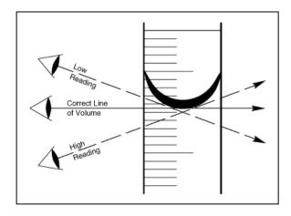
The volume reading is composed of two determinations: The certain digits using whatever marks are on the graduate and the "estimated (doubtful)" digit that estimates one decimal place greater than the smallest marks.
